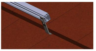
determined, tighten the carriage bolt to 12 lbs-ft.
