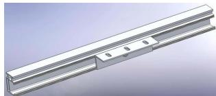
The microinverter mounting kit is designed to bond itself with the rail once it is tightened. The rail nut has teeth along the groves on the two edges and the teeth are pierced into the rail and create bonding between rail and the rail nut. The bolt bonds the microinverter mounting plate with the rail nut. Therefore, the microinverter mounting plate and rail are bonded. Tighten the 5/16" bolt to 12 lbs-ft.
