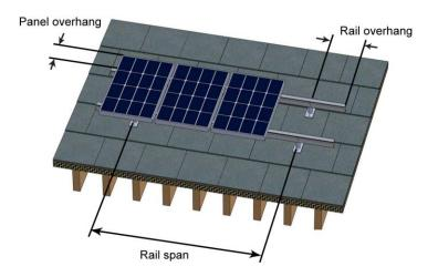
Based on the number of modules, calculate the total length of each row. Remember to add the space for mid and clamps. Add 0.79" for each mid clamp and 0.87" for each end clamp. The total length will be as follows,
