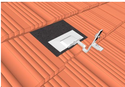
Install steel-roof tile foot on stone-coated steel roof
